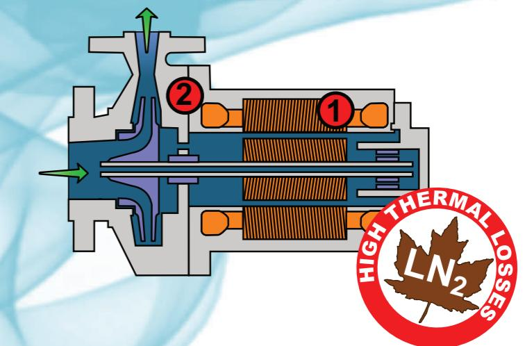
The same remarks are valid for the encapsulated motor version where the fluid is heated by the eddy currents between rotor and stator **3**.
