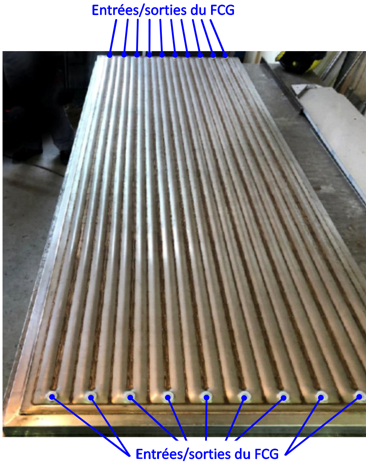
Figure 3 : Ecran Pillow Plate plurimodulaire 3800mm X 925mm (dix modules)
