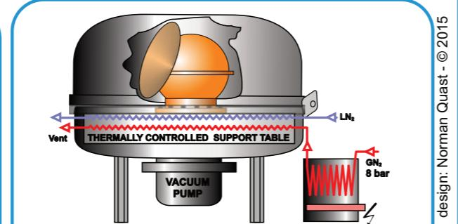
For smaller size vacuum chambers where only a temperature controlled table is required, cast aluminium heat exchangers (see **HEXAL** brochure) can be offered as alternative. Only liquid and hot gaseous nitrogen are used resulting in dramatically reduced
