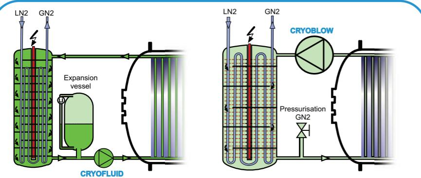
The left heat exchanger configuration with the **CRYOFLUID** is used for liquid heat transfer fluids such as typically silicon oil or 3M segregated hydrofluoroethers (HFEs), while the **CRYOBLOW** configuration on the right is intended for use with gaseous heat transfer fluids (pressurized GN<sub>2</sub> or helium).
